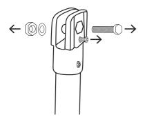
7. Situate the motor head on top of the inner tube, with the holes aligned.
