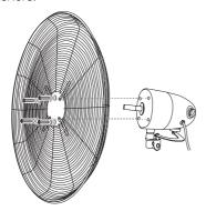
NOTE: Tighten the screws to avoid vibration noise and ensure the grille locking screw and nut are situated at the top of the rear grille.
