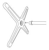
4. From underneath the base, place back the plate and re-insert the washer and hex bolt, using the shifter to tighten.
