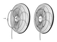
4. Connect the hose connection to the (off) water supply and turn on the fan.
